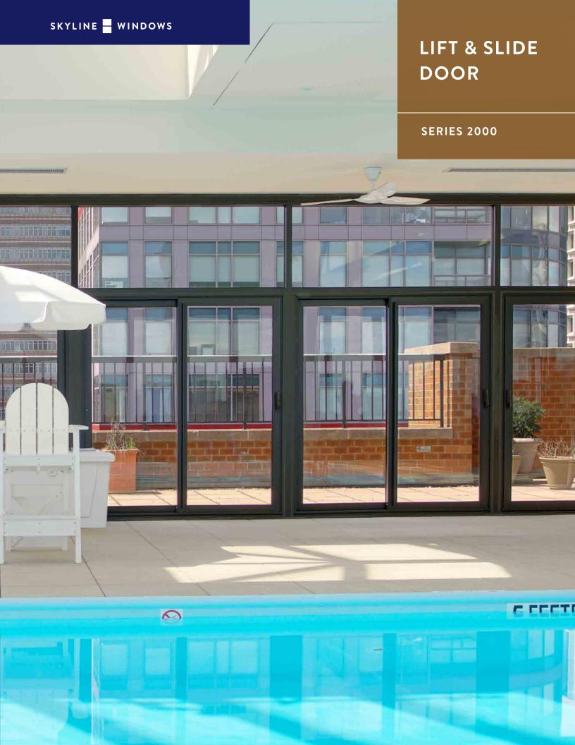
The Skyline Series 2000 Lift & Slide Door is like no other sliding door on the market. The handle rotates 180 degrees, lifting the operable sash off the tracks to disengage the weather-stripping and allow for extremely low friction operation. This unique feature sets the Series 2000 apart from other competitors on the market.
